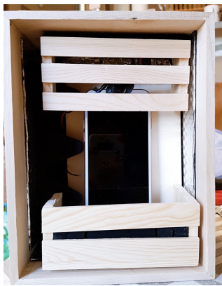
Fig. 8. Our MyBabble prototype consists of a wooden encasing to house a smartphone. Miniature speakers in the prototype are positioned at the microphones of the smartphone. Included circuitry plays MyBabble into the microphones through these speakers.
